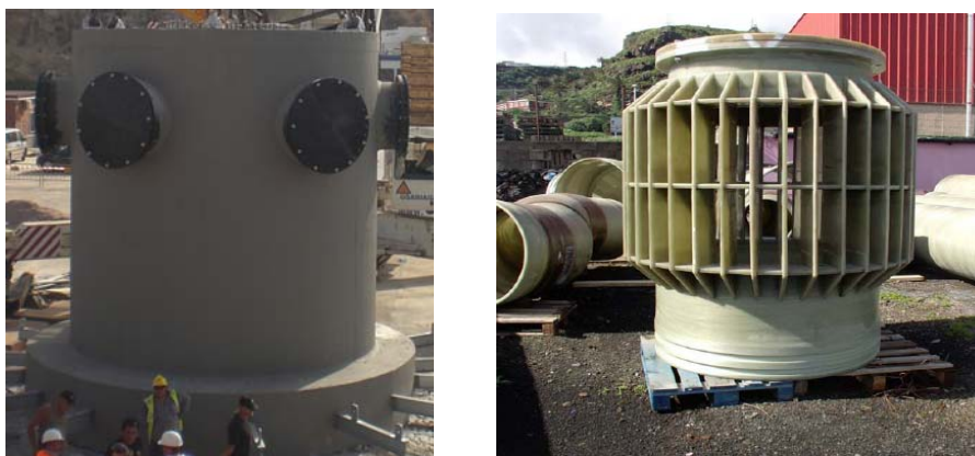
Figure 1: Most habitual types of direct intake structures on the sea bed
